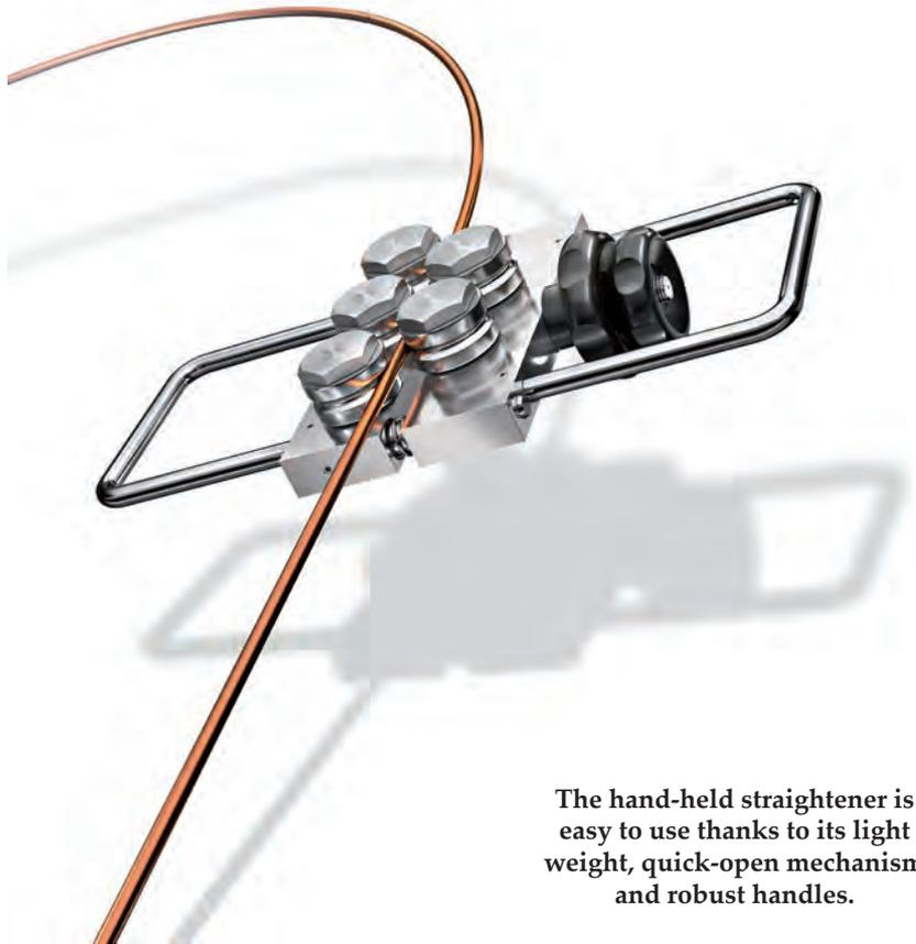
The hand-held straightener is easy to use thanks to its light weight, quick-open mechanism and robust handles.
