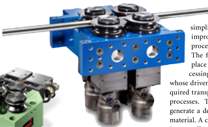
"NADH 160" drive unit for feeding wire diameters greater than 25mm.
