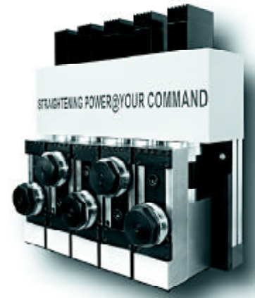
Fig. 2 — Second generation of semiautomatic straighteners (CS EASY LE unit).
