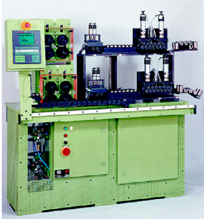
Fig. 1 — Example of the semiautomatic straightening of process materials.
