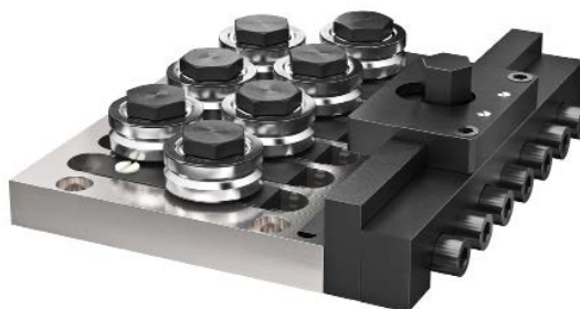
"RTS 7-5.0 4/3" straightener with quick open/close mechanism. Four of the seven rollers are on the operating side. Photos: Witels-Albert
