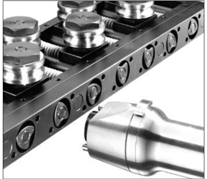
Figure 5: Automatic roll actuators.
