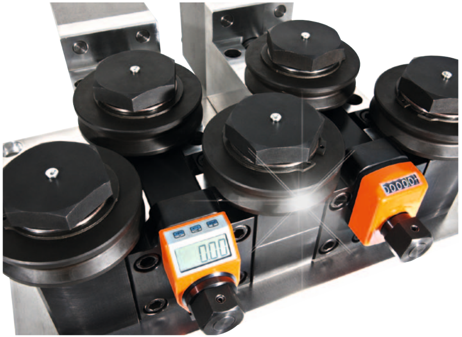
In mass production: five-roller straightening instrument with two Witels-Albert AS 1-20 PO modules.
