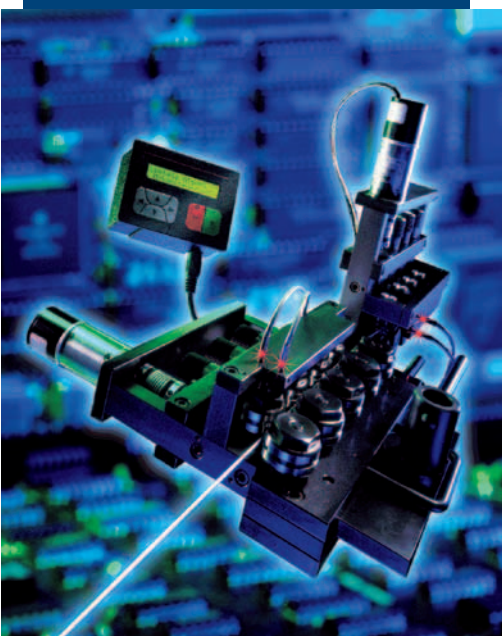
Fig. 2: Semi-automated 2-level straightening system from Witels-Albert
