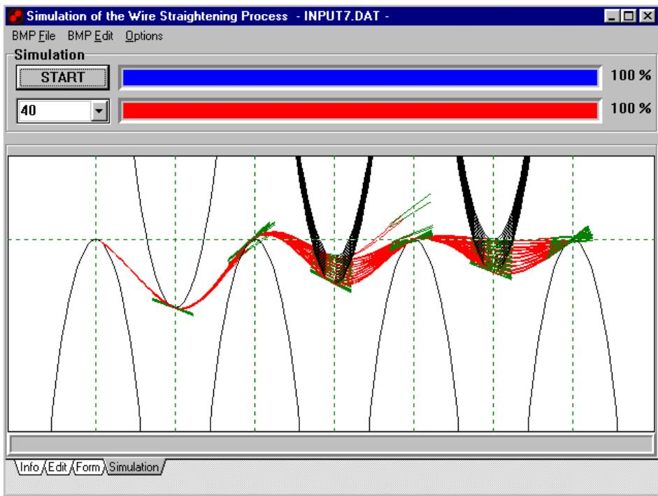
In various processes of metal material deformation there is still room for optimization with regards to the quality of finished product. Straightening on roller straightening units can be regarded as a representative of this group of processes.
